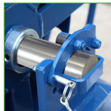
Standard Shaft Safety Locks
