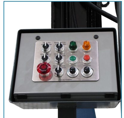
Dual (each column) reel loading controls w/separate free standing operator control pedestal housing full color operator HMI
